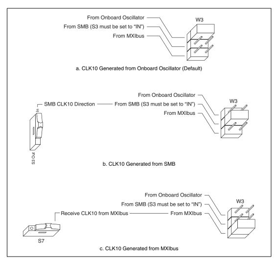
Figure 3-5. VXIbus CLK10 Routing
